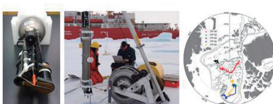
Fig. 1. Left: An ITP end cap fitted with a WHOI-engineered 'bio-suite': a cluster including a commercial triplet fluorometer, an irradiance sensor, and a modified copper shutter for biofouling protection. Middle: A bio-optically equipped ITP being deployed through an ice hole in the Arctic. Right: Sampling tracks of five bio-ITPs operating in the central Arctic and in the Beaufort Gyre between 2010 and 2014.
